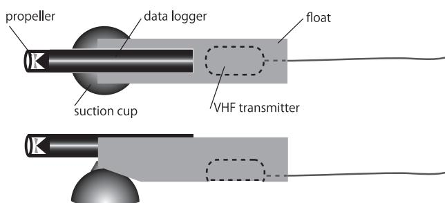
**Fig. 1.** Tag shape used in the current study.
