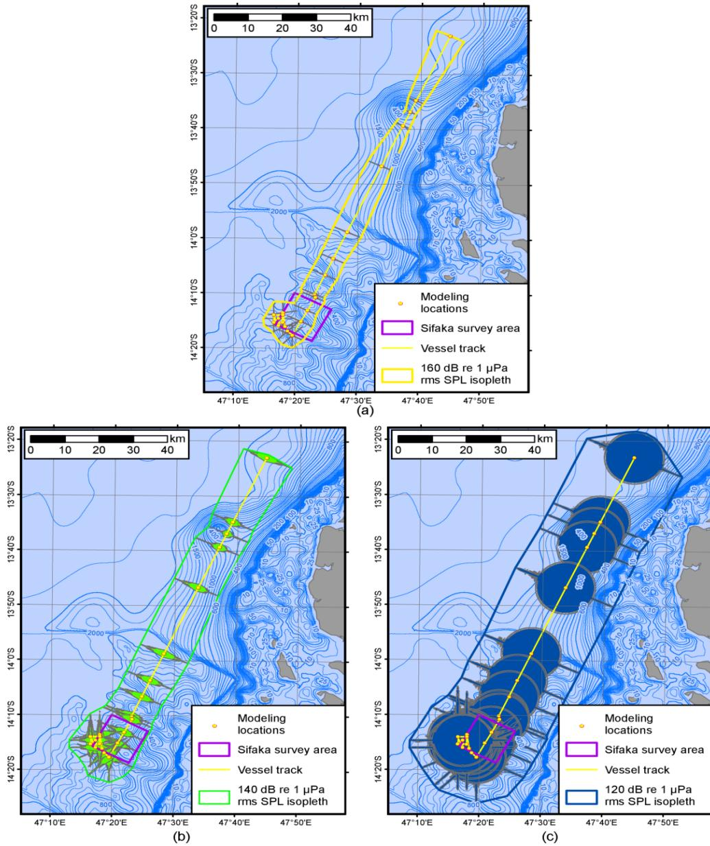
**Figure 7.** Modeled sound levels resulting from *M/V Teknik Perdana*
