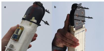
Figure 3. Acousonde tag with (a) three long (6-petal) and (b) three short (3-petal) stainless steel darts and carbon fiber attachment plate.
