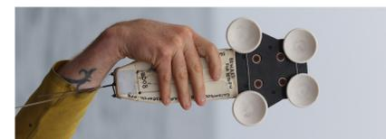
Figure 13. Acousonde tag with tag attachment configuration consisting of four suction cups attached to carbon fiber plate.
