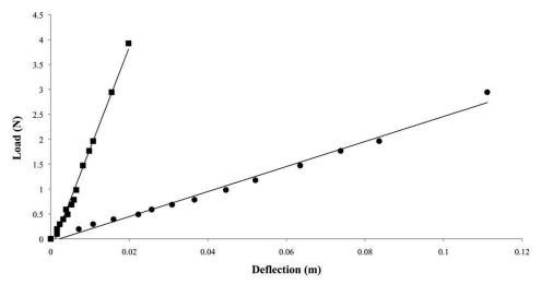
Fig. 6. Load versus deflection plots for the Brown Pelican mandible loaded mediolaterally (circles) and dorsoventrally (squares). Mediolateral line of best fit: y = 25.123x - 0.0565;  $R_2 = 0.98926$ . Dorsoventral line of best fit: y = 204.23x - 0.2386;  $R_2 = 0.98981$ . The slope of
