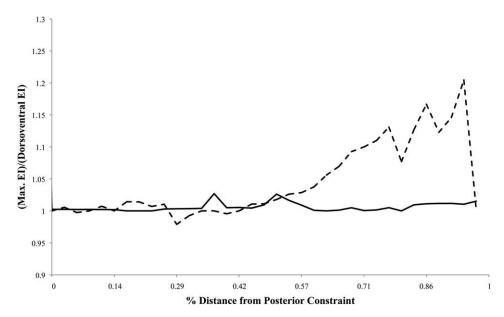
Fig. 5. Ratio between maximum cross-sectional flexural rigidity and dorsoventral flexural rigidity throughout the mandibles of a humpback whale (dashed line) and a Brown Pelican (solid line). The close adherence to 1 in the Brown Pelican indicates that the bone is well designed for bending resistance along its entire length. Values close to 1 are observed at the posterior end of rorqual's mandible, as would
