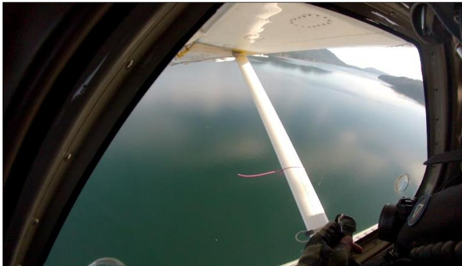
Figure 4. View of transect strip delineated by float and string trailing off wing-strut.
