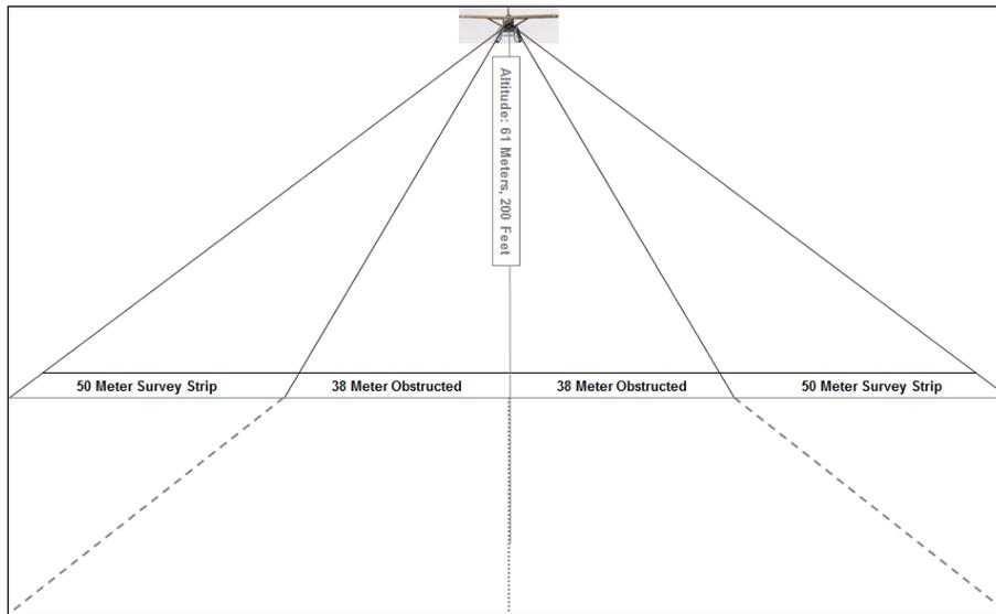
Figure 3. Diagram of left and right survey strips in relation to the transect line. An area 76 meters wide is obstructed from view directly below the aircraft due to the floats. A 50 meter transect strip is viewed from above the floats and out
