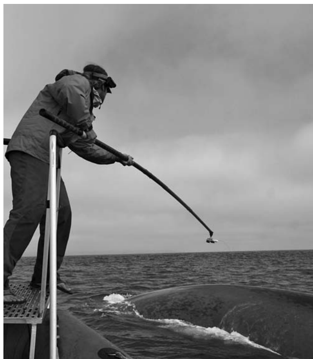
Figure 1. Deploying a suction-cup digital tag to a surfacing blue whale. Photograph: Jeff Foster. The photograph was taken under National Marine Fisheries Service permit no. 14534.
