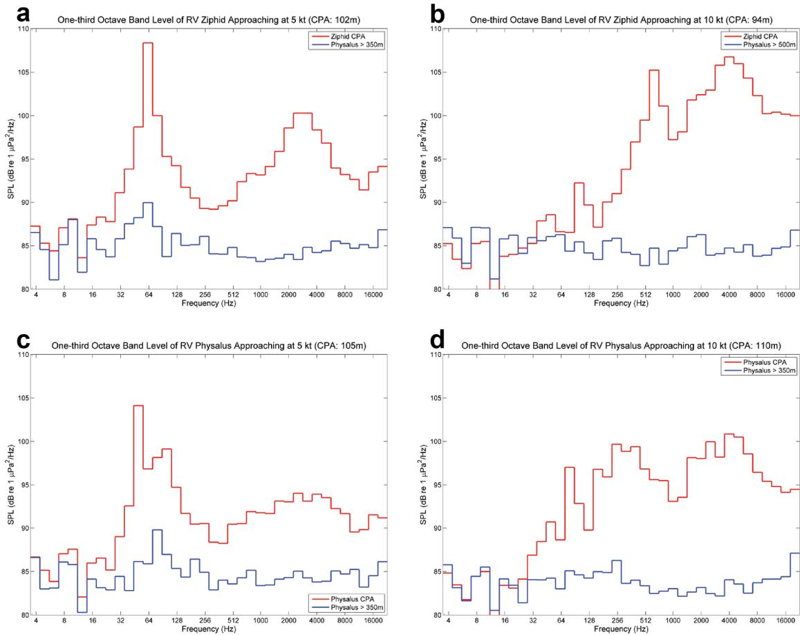
**Figure S1.** One-third-octave band levels for radiated noise from RHIB *Ziphid* during close approaches ( $\sim 100\text{m}$ ) to recording buoys at controlled speeds of 5 kt (panel a) and 10 kt (b) and from RHIB *Physalus* during close approaches ( $\sim 100\text{m}$ ) to recording buoys at controlled speeds of 5 kt (c) and 10 kt (d)
