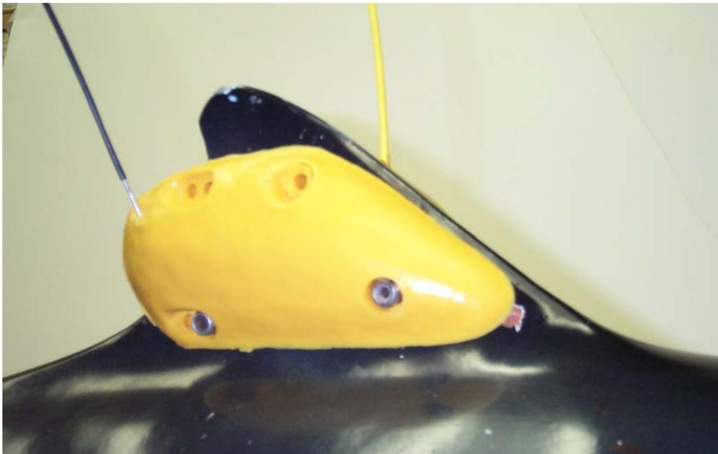
Figure 3.1b. Tag 8 – Paired side mount telemetry tag. Telonics ST-10 left, ATS model 201 right.
