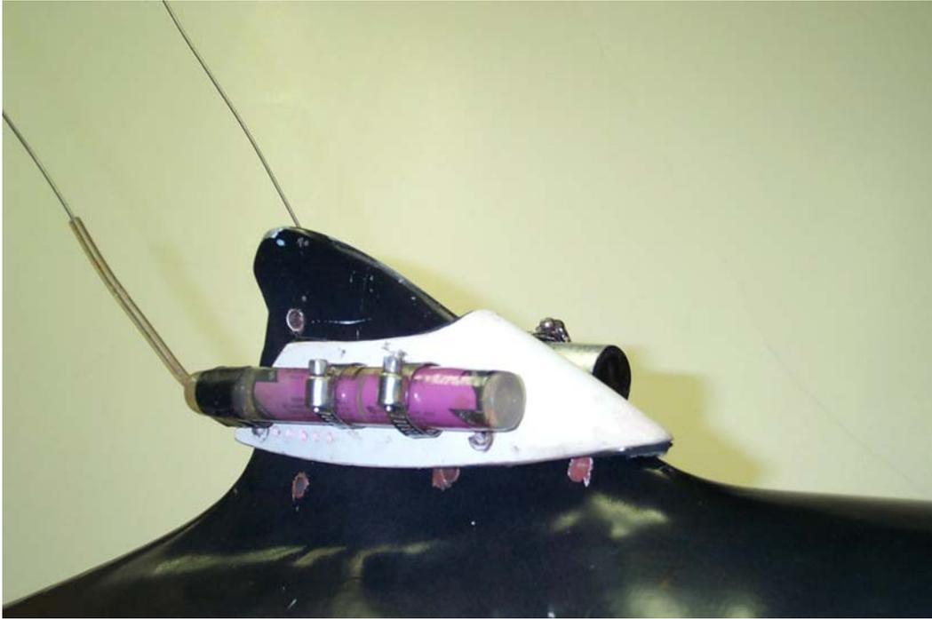
Figure 2.1.a. Tag 1 - dual side mount telemetry tag. Telonics split board ST-10, left side, ATS Model 201, right side.
