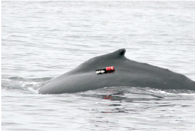
Fig. 1. A tagged humpback whale. The bioacoustic probe was equipped with silicon suction cups for attachment and a flotation device to facilitate recovery.
