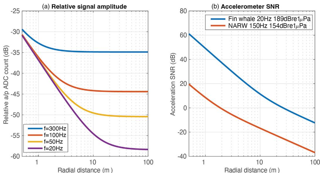
FIG. 1. (a) Theoretical relative amplitudes of digitized signals in a dTag from the accelerometer channels compared to the pressure sensor for a point source. (b) Theoretical SNR for fin and right whale calls on a dTag.
