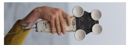
Figure 13. Acousonde tag with tag attachment configuration consisting of four suction cups attached to carbon fiber plate.
